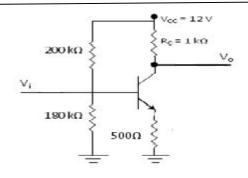
6. The input impedance,  $R_i$  for the CE amplifier shown in the figure below is: Use  $V_T = 26$  mV,  $\beta = 80$ ,  $r_o \rightarrow \infty$
