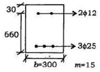
Design a rectangular beam for an effective span of 6m. The superimposed load is 80kN/m and the size of the beam is 300 mm X 700mm overall. Assume effective cover to be 70mm. use M20 concrete and Fe415 grade steel. Use WSM.
