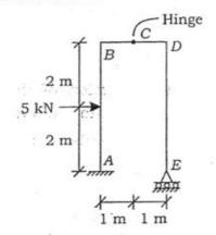
3. Draw the SF and BM diagrams for the frame shown below:
