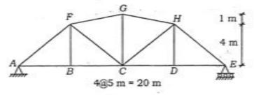
8. Using the method of consistent displacements, determine the reactions of the beam as shown below:
