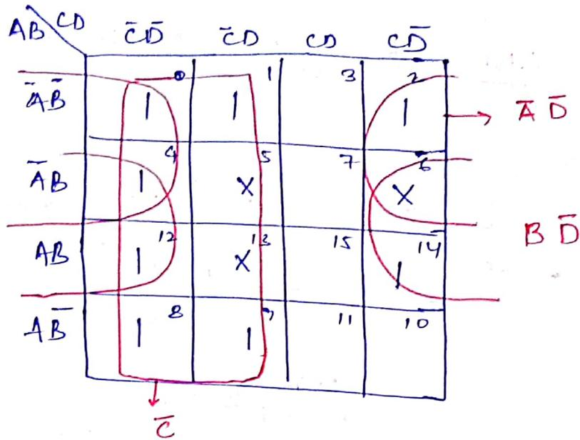
$Y = \bar{A}\bar{D} + B\bar{D} + \bar{C}$
