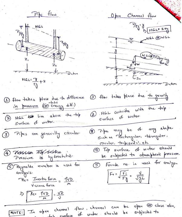
NOTE: In open channel flow, channel can be open & cuse uso but the top surface of water should be subjected to atmospheric pressure (b) Find the discharge in the following channels with a bed slope of 0.0006 and n = 0.016:
