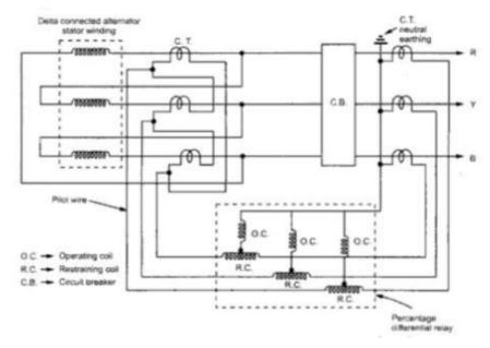
This scheme provides very fast protection to the stator winding against phase to phase faults and phase to ground faults. If the neutral is not grounded or grounded through resistance then additional sensitive earth fault relay should be provided.
