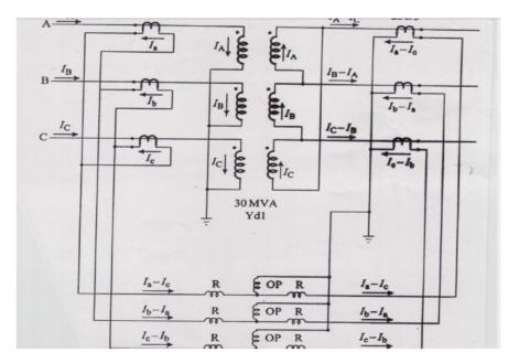
Compared to the differential protection used in generators, there are certain important points discussed below which must be taken care of while using such protection for the power transformers.
