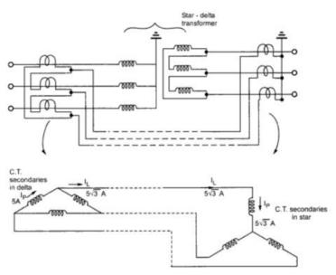
On the primary side, which is 400 V side of transformer the current is 1000 A. Hence C.T.s primary will carry current of 1000 A.
