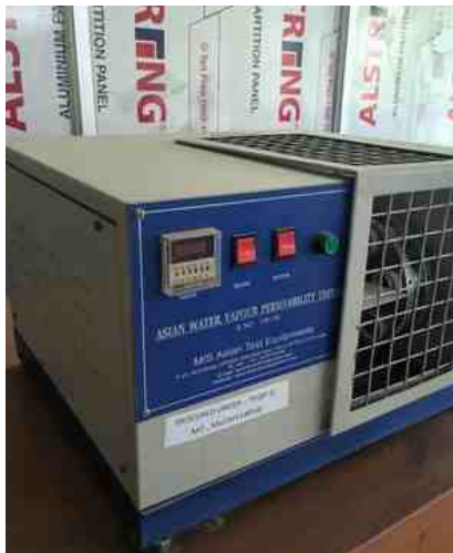
Water Vapour Permeability Tester
